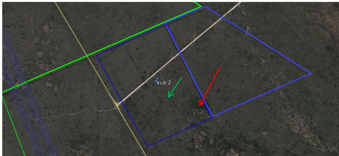
Figure 14: Aerial view of Alternative 2 – note koppie in southeast corner of the substation site (red arrow) and the drainage line (green arrow).
